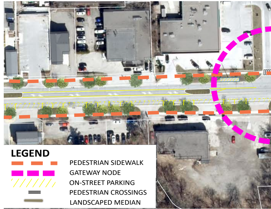
Figure 33: Excerpt of East Broadway proposed improvements in plan view (Broadway at Sherbourne Street)
