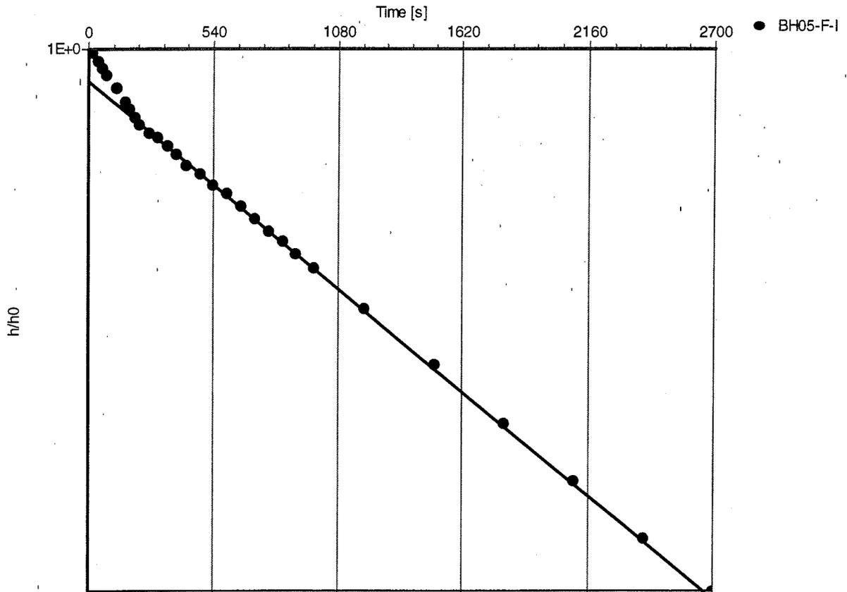
Slug Test: Test on BH05-F-1
